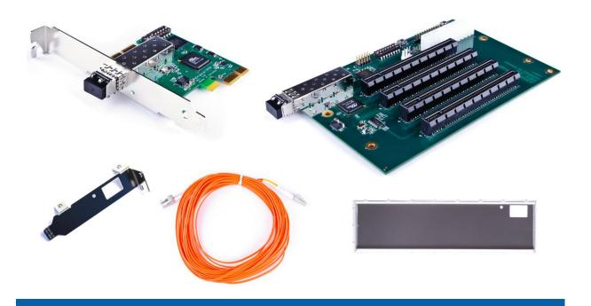
The Adnaco-S1B 5GT/s PCIe Expansion System allows operation of 4 PCIe x1, x4, x8 and x16 cards remotely from the computer system. No additional programming and drivers are required. Any type of PCI Express peripherals can be used including audio, video, graphics, USB, FireWire, SATA, data-acquisition, and network cards.
