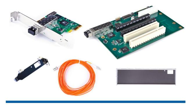
The Adnaco-S1A PCI/PCIe Gen 2 Expansion System allows operation of 2 PCI and 2 PCIe cards over fiber optic cable at distances up to few hundred meters (depending on the types of transceivers and cables) from the host computer system. No additional programming and drivers are required. Any type of PCI and PCI Express peripherals can be used including audio, video, graphics, USB, FireWire, SATA, data-acquisition, and network cards.
