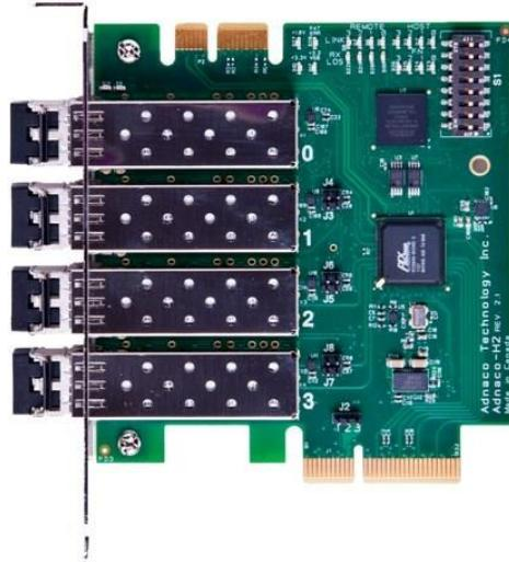
The Adnaco-H2 is a PCIe Gen 2 host/remote adapter, intended to extend the computer PCIe bus over a fiber-optic cable. The adapter is based on a PCIe switch operating in a transparent mode. No additional programming and drivers are required
